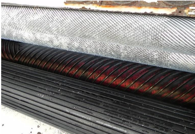
Grip rollers and cutting cylinder.
